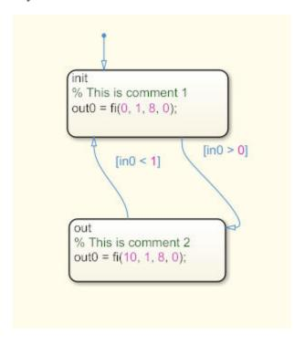
When you generate Verilog code from the model, HDL Coder displays the comments in the Stateflow Chart inline beside the corresponding Stateflow object.
