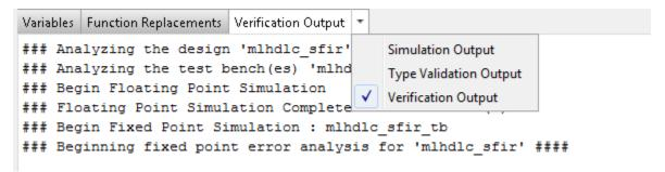
In R2016b, the app displays logs and report links for range analysis and fixed-point conversion on the **Output** tab. It displays logs and report links for verification on the **Verification Output** tab. These tabs are next to each other so that you can more easily find them.
