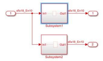
Subsystem1 contains a Subsystem that has a Gain block with the **OutputPipeline** property set to 1 and **ClockRatePipelining** set to on. Subsystem2 contains a Subsystem block that has a Gain block with the **OutputPipeline** property set to 12 and **ClockRatePipelining** set to on.
