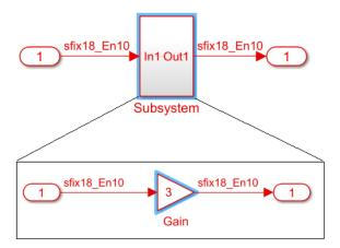
Previously, if you generated HDL code and the validation model for this design, and then simulated the validation model, you observed a simulation mismatch. This mismatch occurred because delay balancing adds a matching delay, which results in the Gain block with **OutputPipeline** set to 12 using one additional latency.
