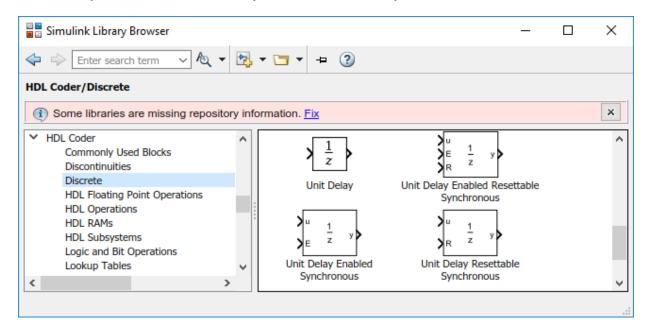
The blocks use the Enabled Delay, Resettable Delay, and the Enabled Resettable Delay block with a **Delay length** of 1 in combination with the State Control block in **Synchronous** mode. The synchronous behavior of the State Control block generates cleaner HDL code and uses fewer hardware resources.
