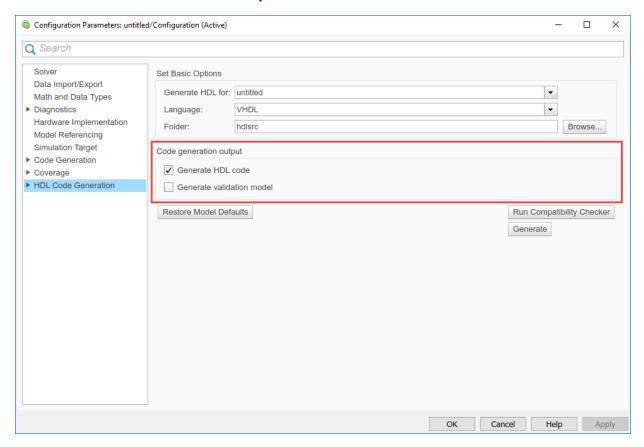
Starting in R2019a, the **Code generation output** option is available under the **Advanced** tab when you select **HDL Code Generation > Global Settings** in the right pane.
