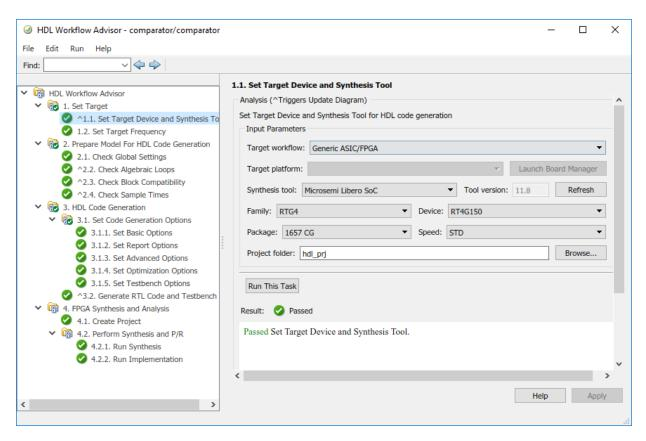
Before you specify Microsemi Libero SoC as the Synthesis tool, set up the tool path by using the hdlsetuptoolpath function. Make sure that you have already installed Microsemi Libero<sup>®</sup> SoC.
