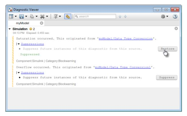
You can also control the suppressions from the command line. To view the existing suppressions on the model, use the Simulink.getSuppressedDiagnostics function.
