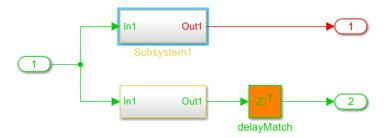
In R2018b, if you enable the **Allow clock-rate pipelining of DUT output ports** setting, the clock-rate pipelining optimization uses different latencies for sampling the DUT output ports. If you now generate HDL code and the validation model for the design containing the Gain block, delay balancing does not insert additional matching delays, which reduces the latency and avoids the simulation mismatch in the validation model.
