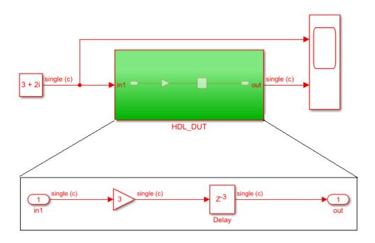
This table displays the generated model when you generate code for the **HDL\_DUT** Subsystem. In R2018b, you see that HDL Coder absorbs the delays as part of the floating-point product operators, **NFP\_mul**. To learn more, see Latency Considerations with Native Floating Point.
